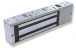
Like the electric strike, these locks can also be set up on a power safe or power secure, however unlike the electric strike, the maglock is constantly drawing power to remain secure. When specifying this type of lock, your installer should be recommending a good back up battery to ensure security is maintained in the event of a power failure.
